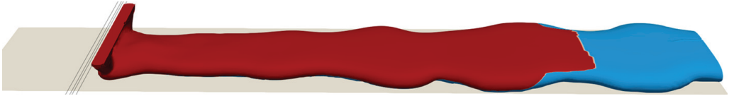
Fig. 6. Phases at t = 2 s with the AC field, current I = 1 kA, frequency f = 4 kHz; red – liquid, blue – solid.
