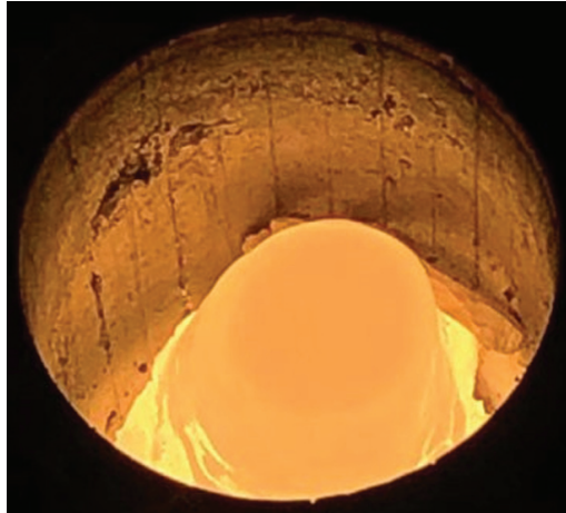
Fig. 2. The induction crucible furnace with cold walls. Source: Institute of Electrotechnology (ETP) of the Leibniz University Hanover.
